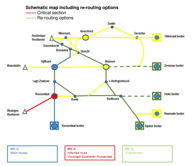
When the route *Vlissingen Sloehaven – Roosendaal (incl.)* is blocked, the sections to be considered for re-routing options are:
