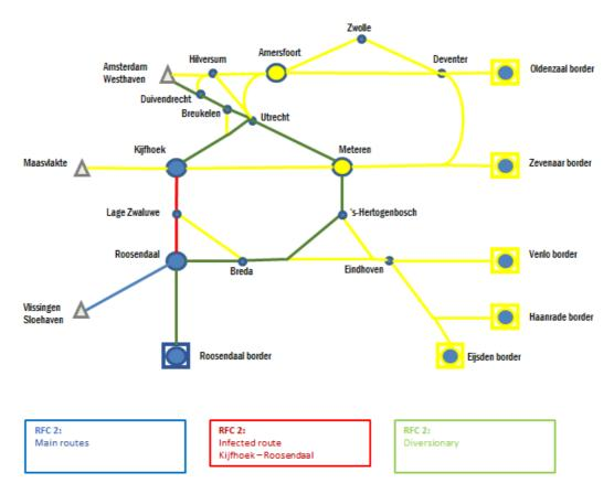
When the route *Kijfhoek South (incl.)- Lage Zwaluwe (incl.) – Roosendaal* is blocked, the sections to be considered for re-routing options are:
