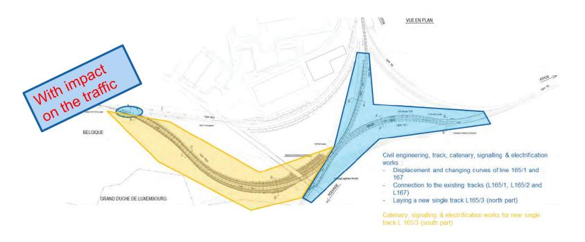
This project takes also the lengthening of 2 tracks to 750 m useful length in the station of Athus (tracks 10 and 11 of the bundle A) into account. This lengthening implies the displacement and renewal of the switches, adaptation of the catenary and signaling
