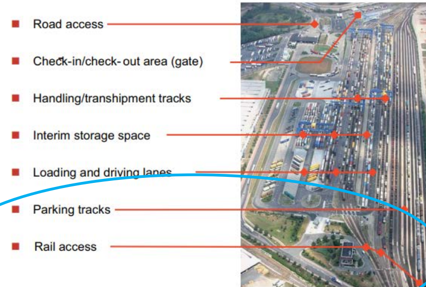
Figure 3-2: Basic components of CT terminals
